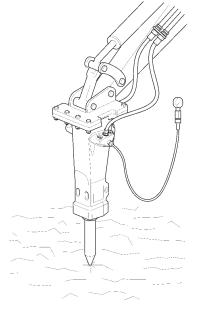
Position the hydraulic breaker vertically towards solid bedrock or similar to adjust the pressure using a pressure gauge.
