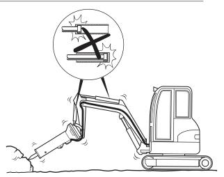
Avoid idling strokes; it causes wear on both working tool and tool retainers.
