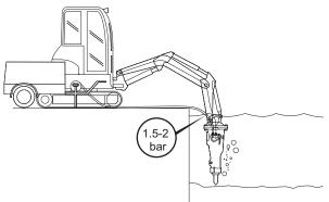
*NOTICE* When operating under water the hydraulic breaker must be fed with compressed air to keep the area between the piston and the inserted tool free from water. If the area between the piston and the inserted tool gets filled with water, it may penetrate into the hydraulic oil system when the hydraulic breaker is started.
