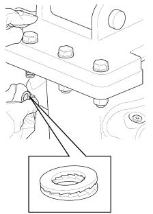
3. Tighten the nuts, see the tightening torque in the table below.
