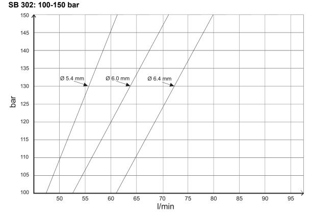
SB 302 Tunnel is delivered with restrictor Ø6.7 for 110 bar operation. As an option, restrictor Ø6.4 for operation at higher pressure, is available.
