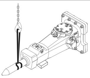
3. Remove and check the lock buffer. Change worn or damaged parts.
