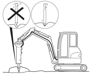
The hydraulic breaker or the working tool is not to be used as a lifting device. When lifting heavy components use the hook on the carrier arm.
