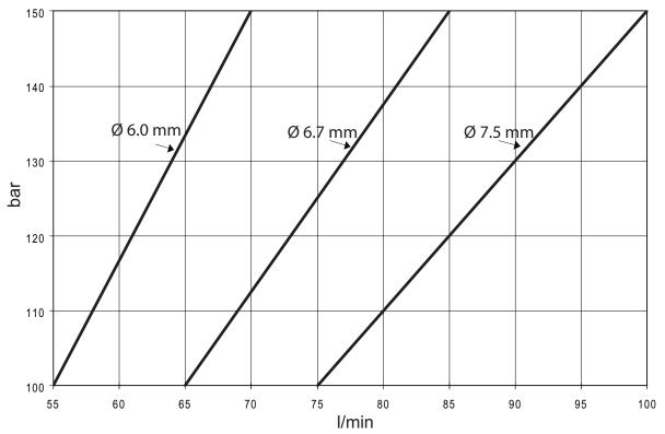
SB 452 Tunnel is delivered with restrictor Ø8.7 for 110 bar operation. As an option, restrictor Ø7.5 for operation at higher pressure, is available.
