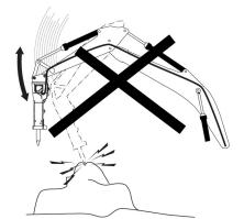
• Never use the hydraulic breaker to move debris.
