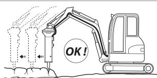
Never run the hydraulic breaker longer then 15 seconds on the same spot. Move the working tool to a new position if the object does not break.
